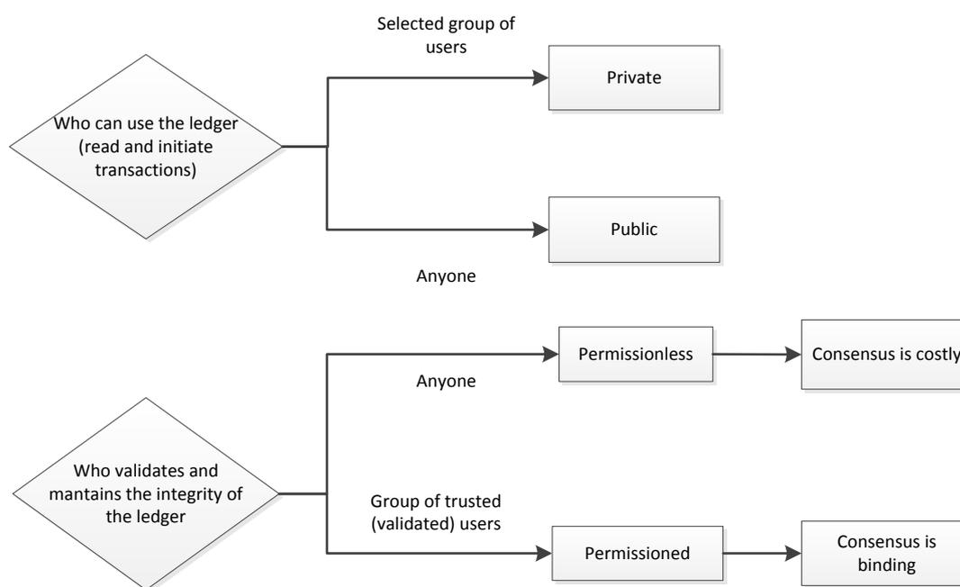
**Figure 2:** Accessibility and validation DL configurations.
